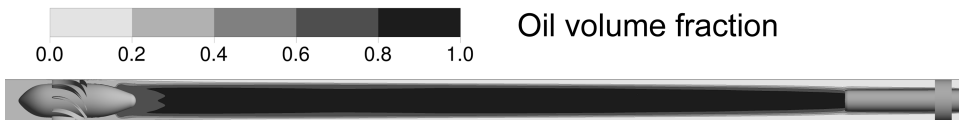
Figure 5.14: Distribution of time-averaged oil volume fraction \alpha on plane through the axis of the separator. Large hold-up of oil is seen and maximum \alpha is just above 0.80. FS = 0.30, \text{Re}_D = 0.86 \times 10^5 , Sw = 6.61, d/D = 1.00 \times 10^{-3} , \alpha_{inlet} = 0.25 .
